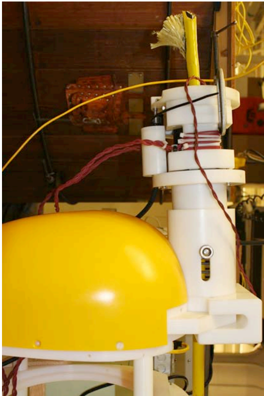
Figure 2. The inductive power system coupler
