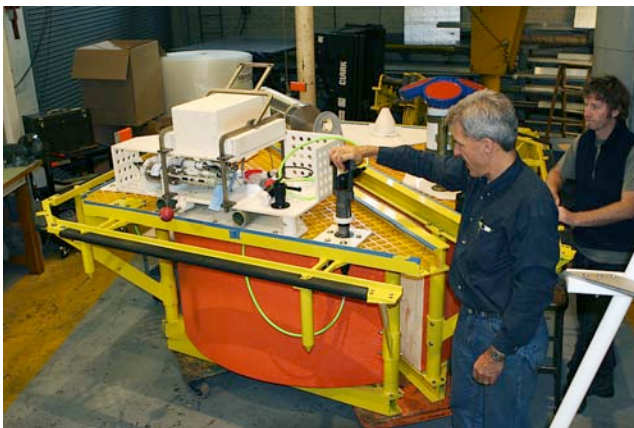
Figure 3. The subsurface float and secondary node, with instrument package and ADCP
